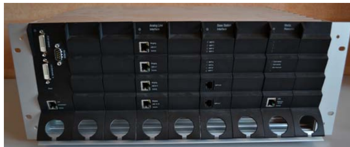
Figure 2 Spectralink DECT Server 8000 Chassis with CPU (with Link option) and Interface cards
