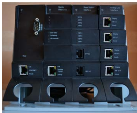
Figure 3 Spectralink DECT Server 2500 Chassis with CPU (without Link option) and Interface cards
