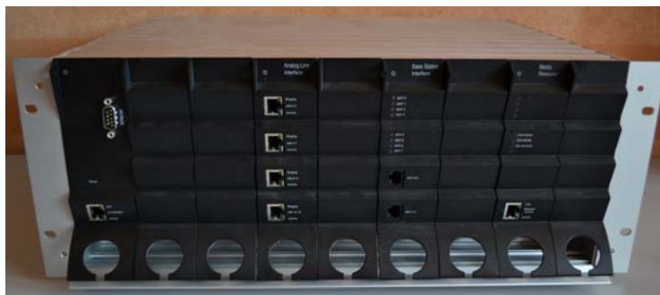
Figure 2 Spectralink DECT Server 8000 Chassis with CPU (with Link option) and Interface cards
