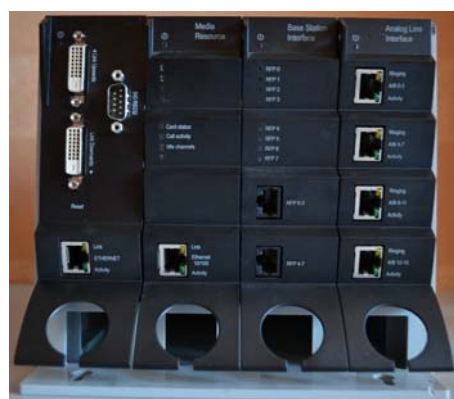
Figure 4 Spectralink DECT Server 2500 Chassis with CPU (with Link option) and Interface cards
